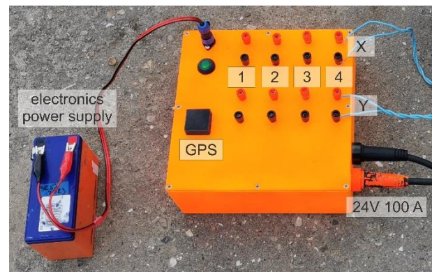
Figure 4. Prototype current transmitter for creation EM signal in the AMT dead band
