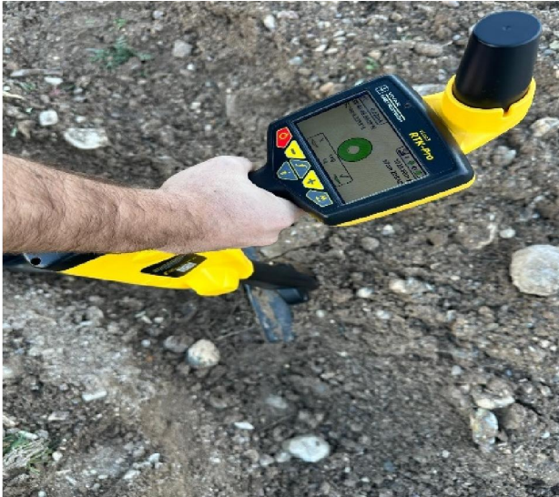
Figure 1 RTK-Pro Receiver and transmitter unit
