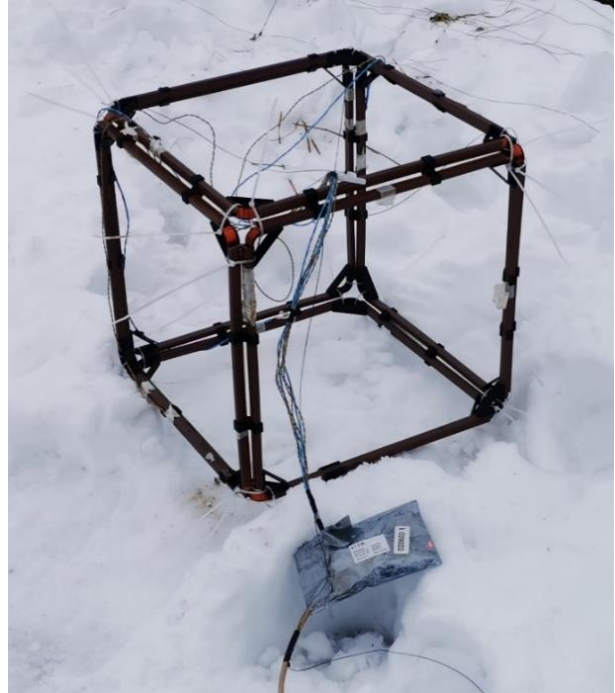
Figure 1. Cubic sensor prototype with dimensions of 45 x 45 x 45 (cm) for 3-component magnetic field measurements at frequencies from ~1 to ~30 kHz.
