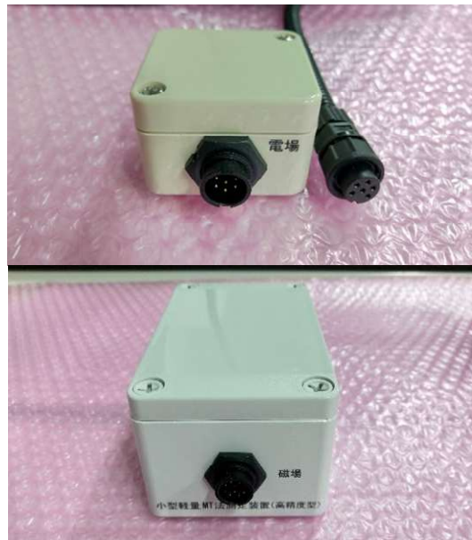
Figure 3. Photos of the electric sensor module (upper) and magnetic sensor module (lower) for C3.
