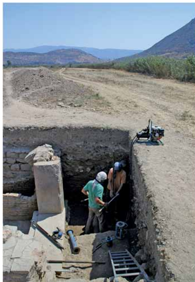
Figure38. Vibracoring in the necropole at the flank of the canal connecting the Roman harbour with the sea. The coring at a grave of the necropole dating from the 3 rd century AD (oral comm. by Dr. Steskal) is part of a new project which aims to clarifying the building phases of the canal and its final siltation. The persons are extracting the drill cores. The green reeds in the right part of the photograph mark the area of the canal. The theatre of Ephesus is visible in the background.
