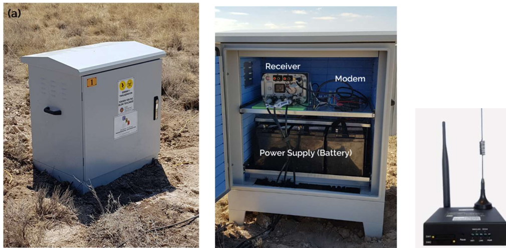
Figure 2. a) MT measurement system box designed in accordance with the field conditions, b) the layout of the system inside and c) the modem used.
