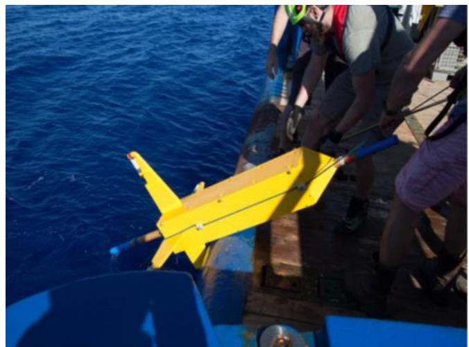
Figure 1. Left: Golden Eye recovery on RV Pelagia. Top: Vulcan E-field receiver being deployed at the aft deck.
